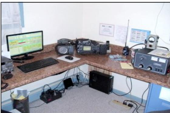
This view is of my Icom 746Pro and rotor box. On top of rotor is my Jetsteam 222 rig. On top of 746 is my MFJ Voice Keyer. Came in real handy on January Contest Sunday when contacts slowed down. On top of rig supply is a SignalLink USB for working digital modes. Also seen is my Ameritron 811 Amp 600 watts out for the low bands. PC & UPS under the counter-top.
