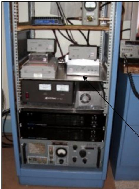
The rack all wired up and in place. The bottom is the AM-6155 amp. Above that are 2 – GlenAyre 28v 25amp power supplies. Above that on left is an Astron RS35M 13.8v 25amp supply. On right is a Power Source 13.8v 75amp switching power supply. Above that is 903 & 222 transverters with sequencers and power amps. Above that is a Teletec 432 amp that puts out 150 watts.
